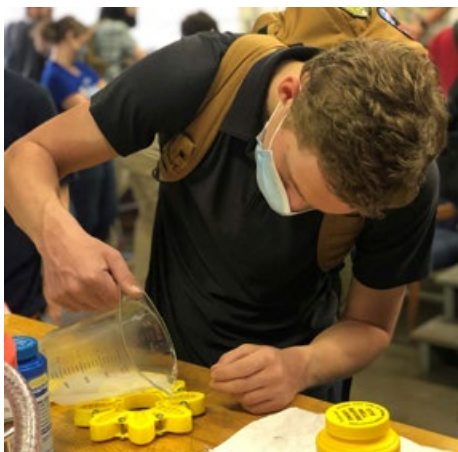
SEAP Intern Ian Clark pours silicone mix in a SeaJelly mold while on tour at Carderock in West Bethesda, Md., on Aug. 4, 2021. In each piece of the material is what Nunes calls a "void," which each have chambers inside. Four pumps and four actuators pull in water and fill the tentacle-like arms, allowing the vehicles to swim underwater. (U.S. Navy photo by Edwin Hernandez)
